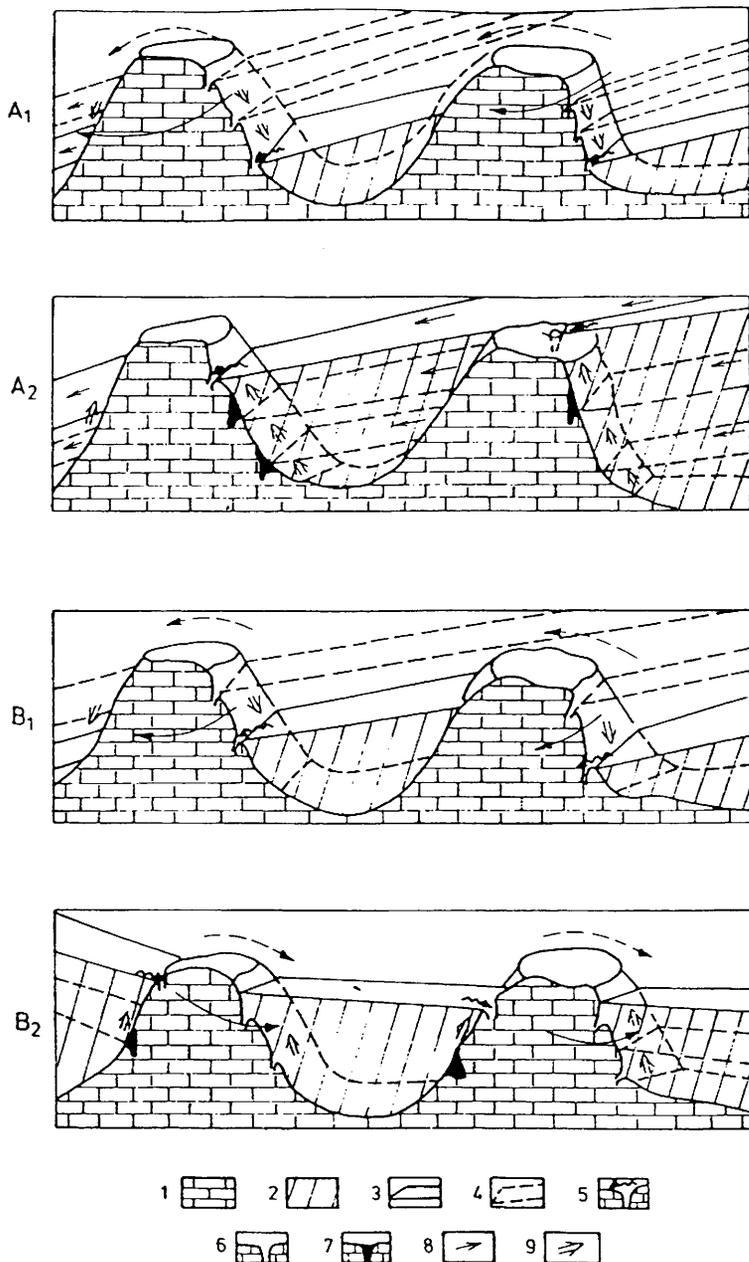
Fig. 46. Karstification of paleokarst elevations during exhumation (A<sub>1</sub> and B<sub>1</sub>) and burial (A<sub>2</sub> and B<sub>2</sub>)
