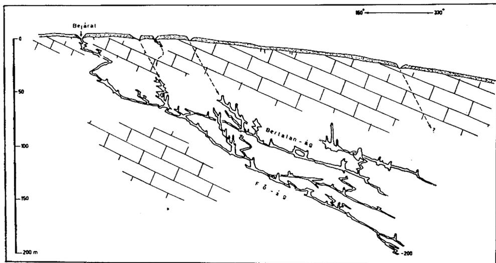
Fig. 12. Longitudinal section of the Alba Regia Cave (after KÁRPÁT 1982). Vertical sections of passages are probably chimneys formed by recent karstification and their extension is from the already existing main branch due to the effect of infiltrating water
