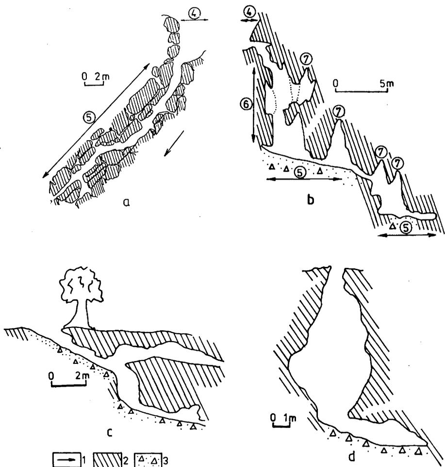
Fig. 7. Simple chimney (a) in doline-with-ponor G-5/a, composite chimney (b) in doline-with-ponor Ho-1 (Homód-árok area) and truncated chimneys in the Gyenespuszta cave (c) and Cseresi-zsomboly aven (d) (surveyed by KÁRPÁT 1977, figures b, c and d are from Reports for 1978, 1979 and 1984 of Cholnoky J. Caving Group)
