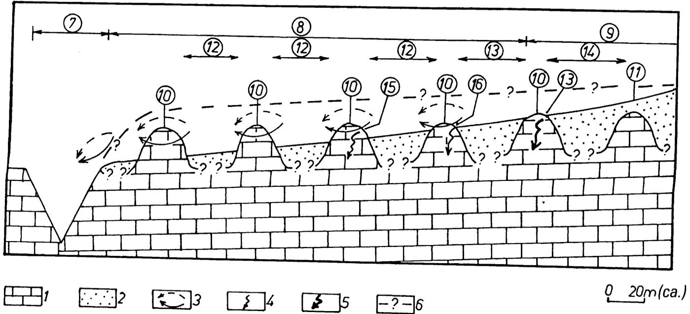
Fig. 47. Denudation of slightly tilted block through sheet wash (the greater is the extent of tilting, the more intensive the removal of cover sediment is, even in lack of a marginal valley)
