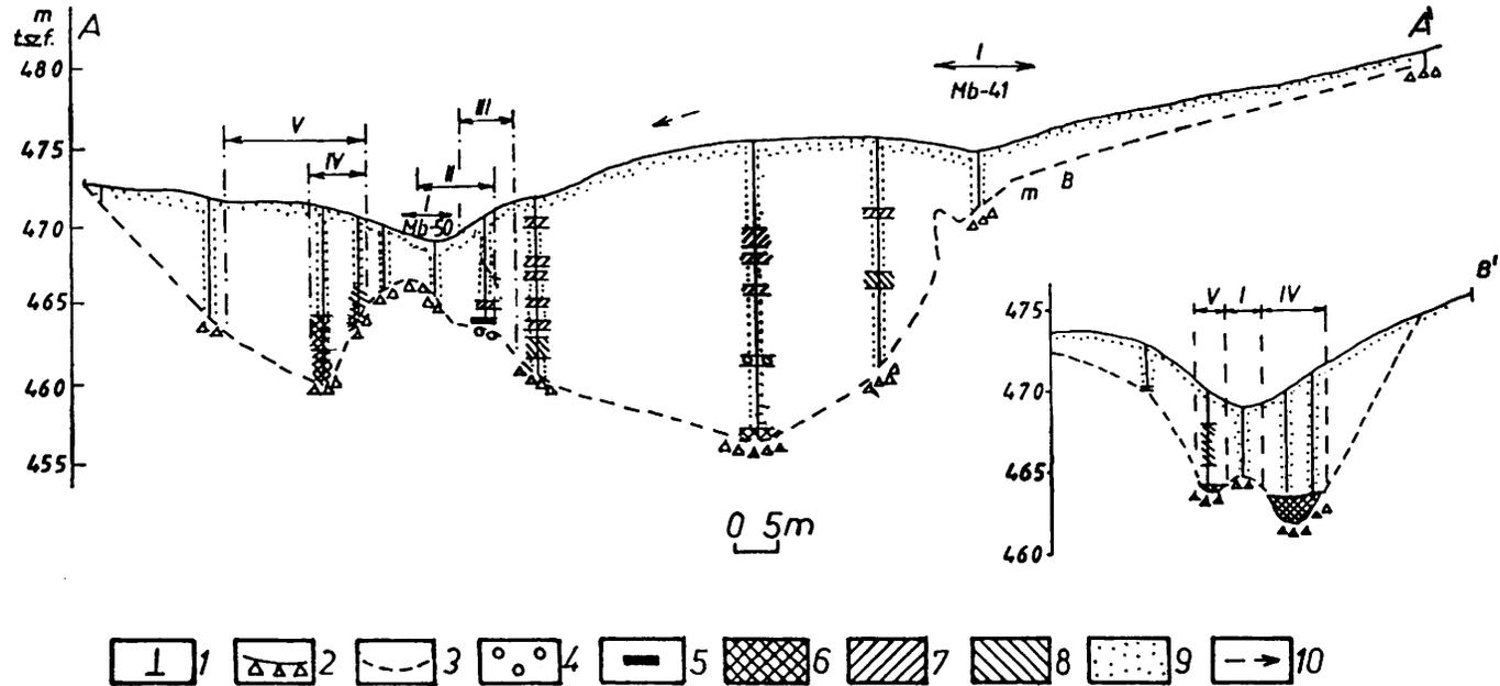
Fig. 45. Structure of carbonate basement and cover sediments in the area of the pseudodepression near karst object Mb-50 (Mester-Hajag)
