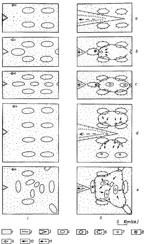
Fig. 17. Development of pseudodepressions of various morphology during exhumation of the broader environment through stream erosion
